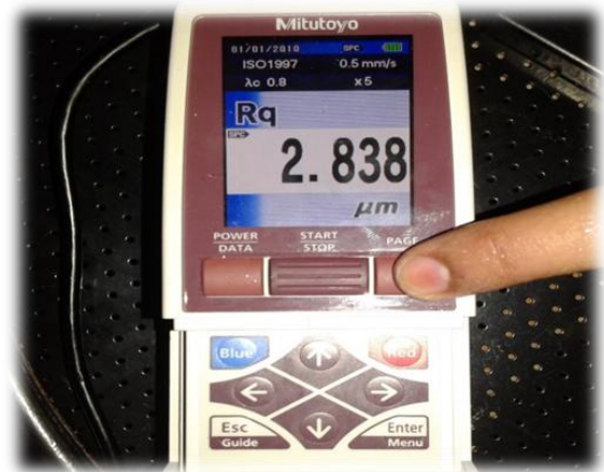
Figure.2: MITUTOYO, SURFTTEST SJ.210 used for measurement of surface roughness
